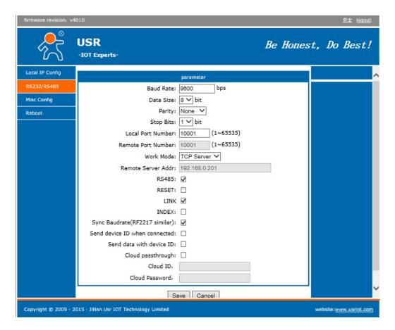
1)set baud rate to 9600 and local port to 10001, and net protocol set to "TCP Server" then save and reset.(this is already done by us initially when tested in house)
