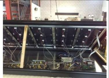
Sign Hinged Open (For service purposes only). Allan Keys in bottom of face MUST be accessible for service.
