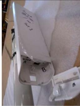
NanoStation #2-Wifi Bridge at Sign. To be Mounted at sign closest to the building. "Line of Sight" to the building is required.
