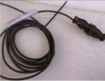
Interconnect cable between Master and Slave Sign must be screwed tightly together and "Clicked" into place.
