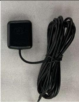
GPS to be installed with Line of Sight to the sky/satellites - external to the sign.
