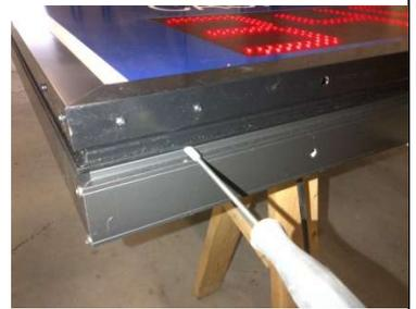
Allan Keys loosen to open and service sign. Require access from the top and bottom of the sign face.
