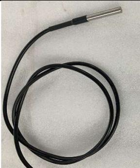
External Temp Sensor-not to be in direct sunlight, or directly installed on dark surfaces to avoid radiant heat-external to sign.
