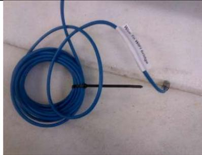
NanoStation #2-Wifi Bridge Cat5-POE-Connection from the back of the Master sign. Must be connected at time of Instalation to avoid damage to wire with power on it
